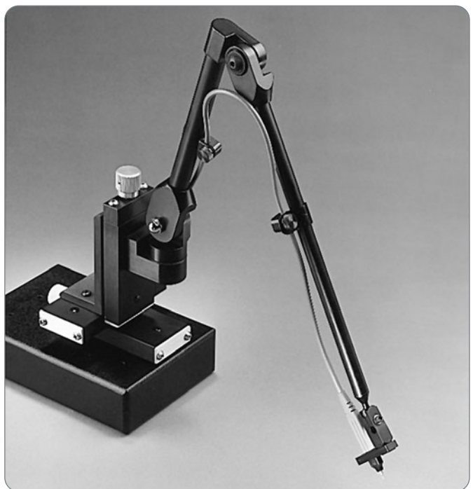
► Figure 2-10. Example of a probing station designed for probing small geometry devices such as hybrid circuits and ICs.
